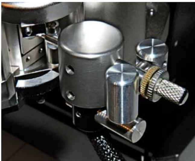
Lock it in place with the left end (pointing towards the AXIOM's bearing) barely visible outside the POM block and the right end extending towards the rear by almost half of the length.
