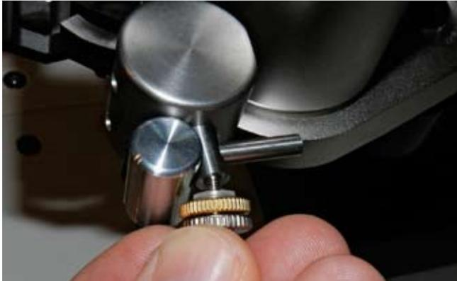
Next please slide the other small cylinder onto the free part of the short shaft. Do fix it in place - right at the end of the shaft, so that the shaft ends with the cylinder - with the small M3 invert Allen screw.
