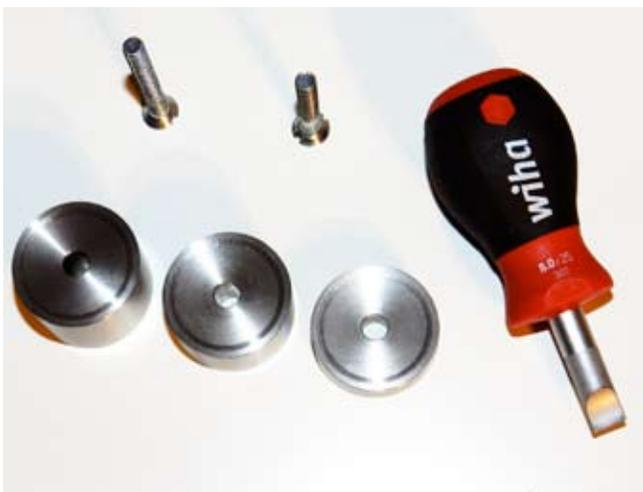
Now do take the (3) hardened stainless steel washers. Select the one most likely to elevate the AXIOM to a suitable horizontal position relative to the turntable platter's surface.
