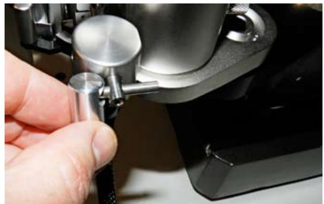
Please do insert it with the fixed cylinder - which is firmly attached to the shaft - pointing outwards, away from the turntable platter and the AXIOM's main assembly. Now do move the cylinder as close as possible to the main shaft.
