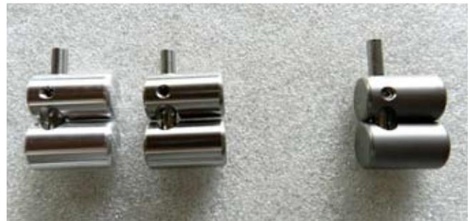
One of the 2 cylinders features an Allen screw. Undo this screw and slide the cylinder off the 4 mm shaft. This 4mm shaft is firmly attached to the other cylinder. Take the shaft with cylinder and insert it through the horizontal hole at the end of the shaft carrying the counter balance weight.
