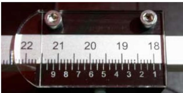
This is 215,25 mm P2S - for the DaVinci 9" tonearm. Note that the white line between "2" and "3" is in-line with the black line above on the aluminum scale. This means 215 mm PLUS 25/100 mm. Resulting in 215,25 mm P2S. The vernier scale "adds" the 5/100 mm value to the full mm read-out on the large metric scale.
